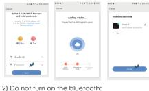
Select "Universal Remote Control" from "Others" enter into the Wi-Fi password, make sure the LED indicator is blinking rapidly, if not, please open the stand at the back, hold the reset button for about 5s till indicator blink quickly, it will connect. ® ® № 33% ® 21:59
